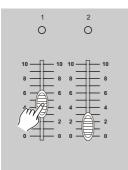
3. Create a desired scene using Channel Sliders 1-24. At 0% or DMX 0, these sliders should be at 0 position, and at 100% or DMX 255, these sliders should be at 10 position.
